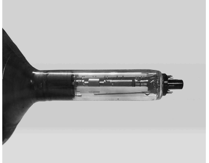
A spare Conrac cathode ray tube that can replace the one used in Magnet TV in case of damage or wear
